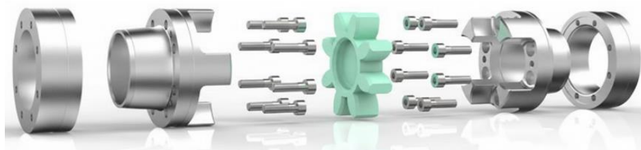
Type 2.5 clamping hub double slotted, without feather keyway
